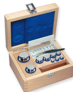
Wooden case, lined, for weight sets, knob shape
