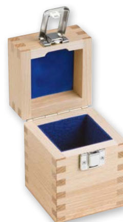
Wooden box, lined, for individual weights ≥ 1 kg
