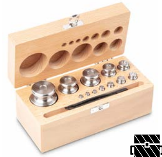
Wooden case, for weight sets, knob shape, finely turned stainless steel
